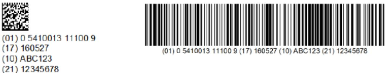
Figure 2.2 GS1 DataMatrix and GS1-128
